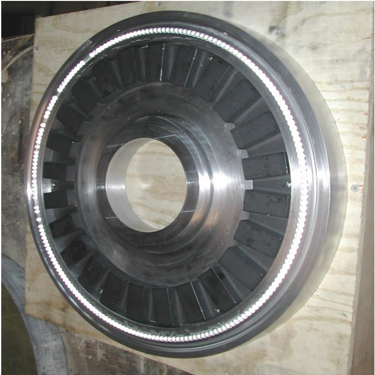
This is the rotor, which is stationary for the azimuth assembly. Notice the precision glass balls for the ball bearings. They need to be non-magnetic or they just hop over to the powerful, rare earth magnets.
