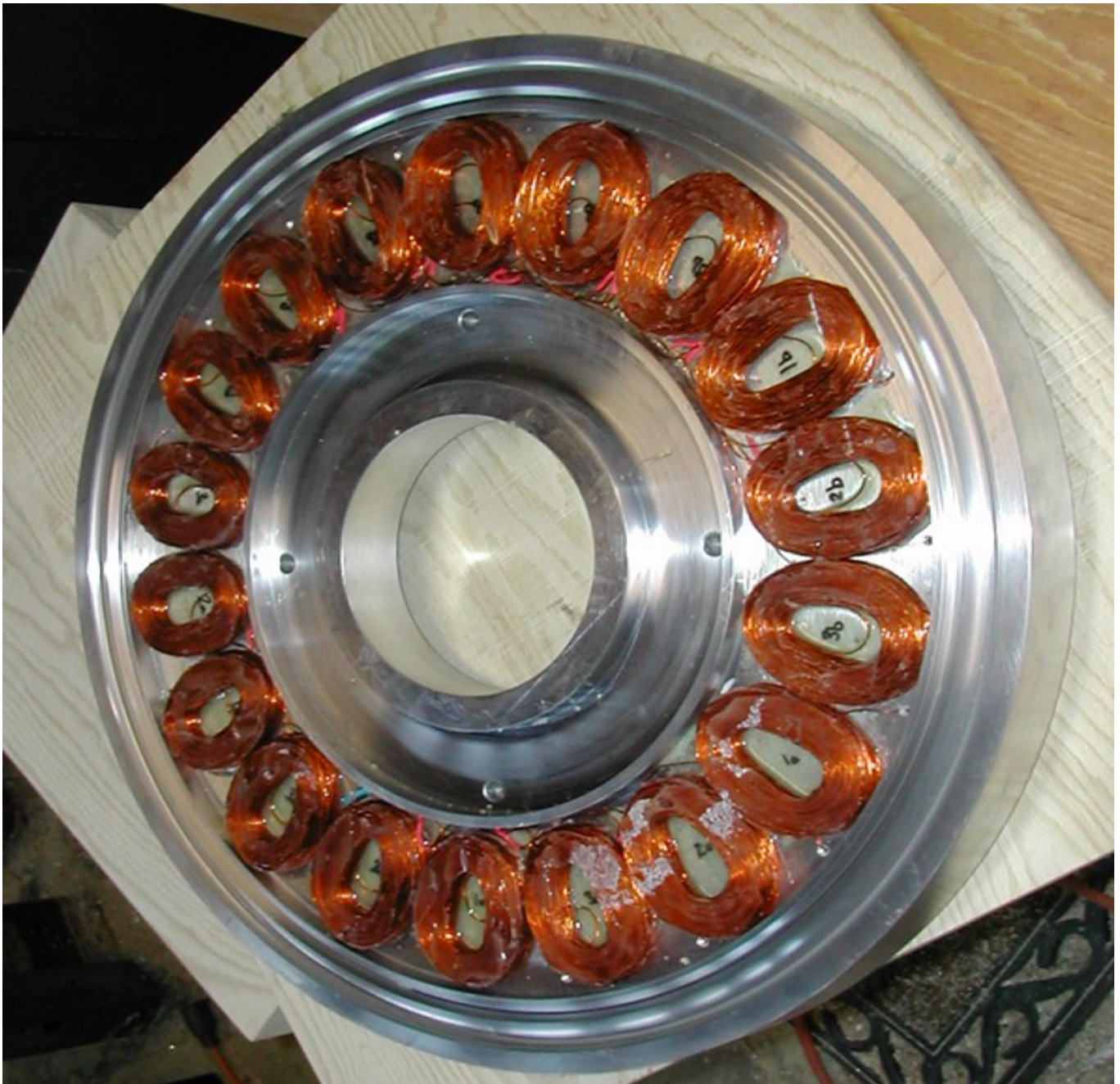
This is the stator and top half of the azimuth bearing assembly that Dave Rowe designed and fabricated.
